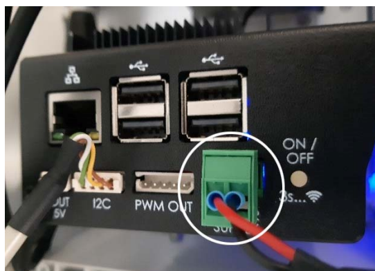
Figure 2–14 – Connection of the 2-pin connector to the 8-30 VDC IQ-LINK input
