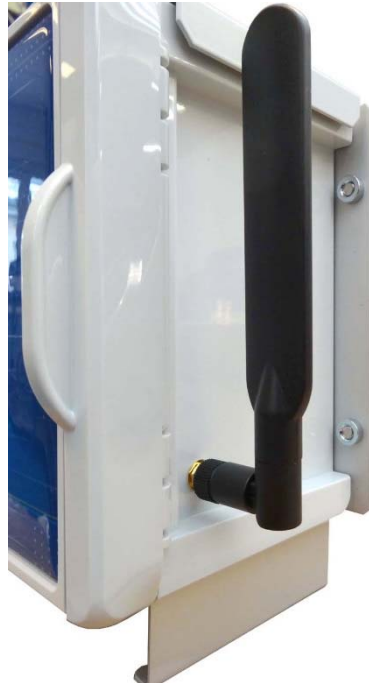
Figure 2–2 – Radio antenna of CAIRNET
