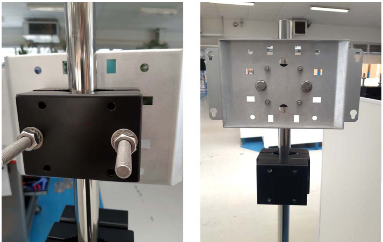
Figure 2–15 – Fixation of CAIRNET holder and solar panels to the tripod mast
