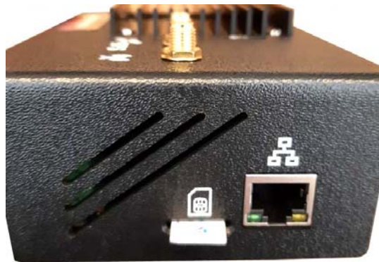
Figure 2–8 – Micro SIM card insertion
