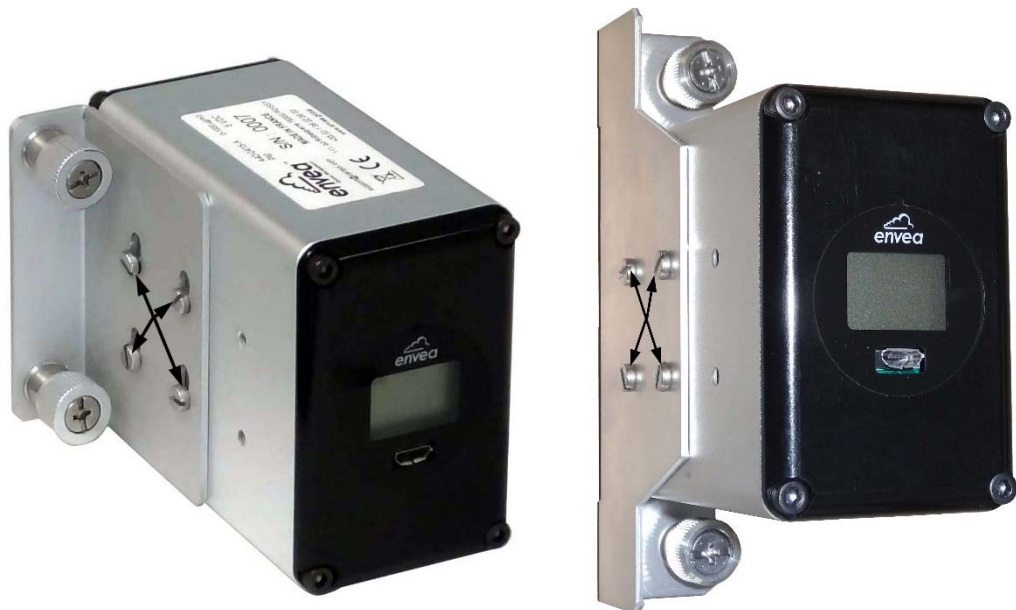
Figure 2–4 – Screwing the angle bracket on the CAIRSENS
