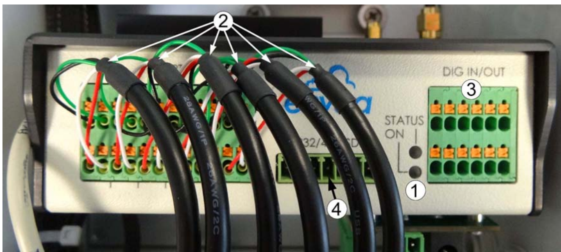
Figure 1–5 – IQ-LINK front panel
